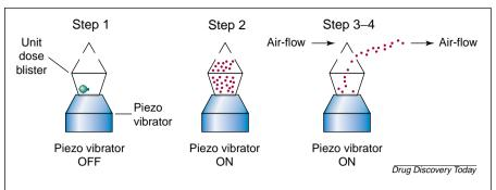
Figure 1. Principle of operation of the MicroDose dry powder inhaler. In step 1, the piezo vibrator is off and the drug is aggregated in the blister. In step 2, the high frequency piezo vibrator deaggregates the powder into its primary particles while still in the blister. In step 3, the deaggregated particles circulate to the top of the blister where they are forced out through pierced holes into the airstream. In step 4, the user's breath carries the drug powder to the lungs for absorption.
